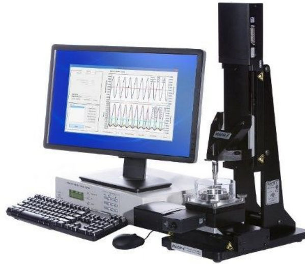
Figure 7. Illustration of Mach-1™ set-up. Mach-1™ for mechanical compression is connected to a PC and controlled using Mach-1™ Motion software. Samples are loaded onto the Mach-1™ platform and compressed by a transducer. Transducer signals are sent to the PC for data logging and profile plotting.
