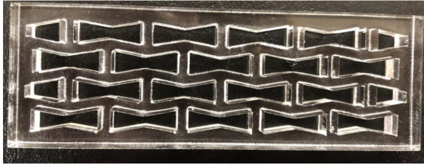
Figure 15: Re-entrant Masters-Evens model 1 acrylic Top view of a laser cut mold of the Re-entrant Masters-Evens model 1
