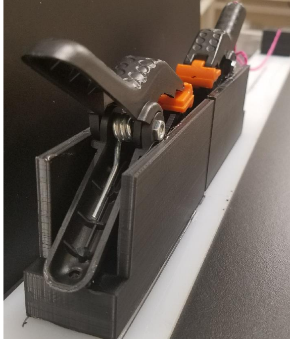
Figure 23: Angled view of clamp set-up Shows clamp set-up for testing weights and the pink yarn being guided in the black block before going off the table where it is attached to the desired weights
