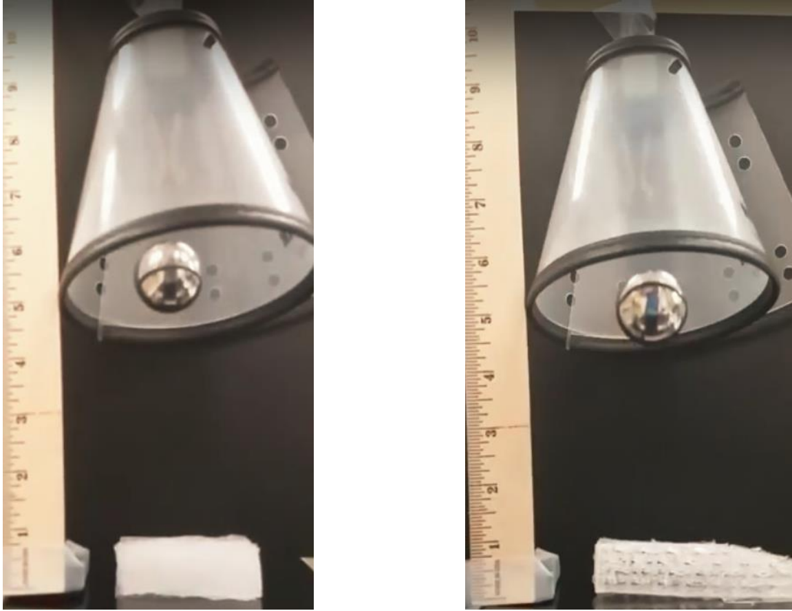
Figure 30: Shock absorption testing on the left is the non-auxetic polyurethane structure that on average had a final height of 5.56” when dropped from 9.5” and on the right is the auxetic polyurethane structure that on average had a final height of 4.88” when dropped from the same height
