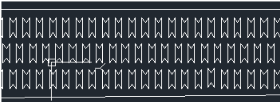
Figure 8: Re-entrant Masters-Evans model 2 drawing This design was created in SolidWorks and has a high maximum area expansion when comparing various auxetic patterns
