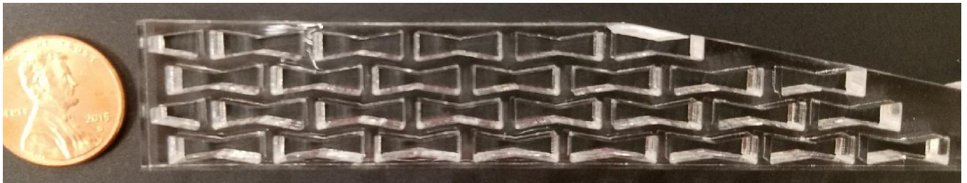
Figure 10: Final auxetic heel support acrylic This is our final auxetic heel support structure created. It is the same dimensions as the rectangular piece above, but slopes downwards at the bottom for additional comfort. It is the model 1, small polyurethane structure
