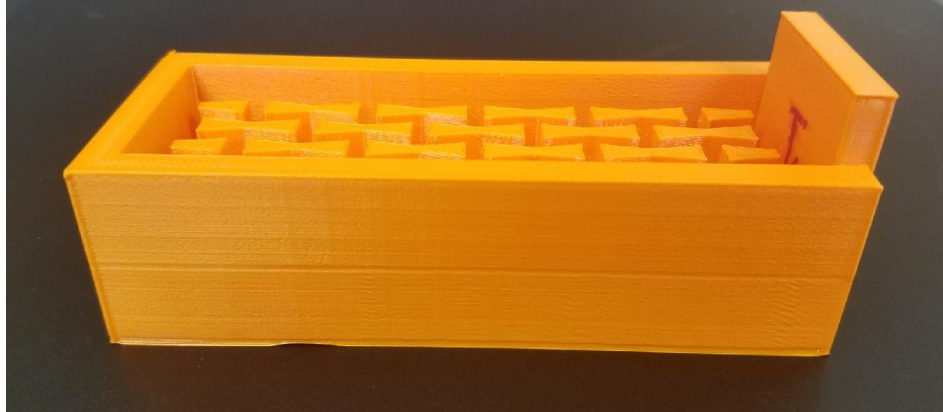
Figure 12: 3-D printed side view model 1 Side view of a 3D printed mold of the Re-entrant Masters-Evans model 1
