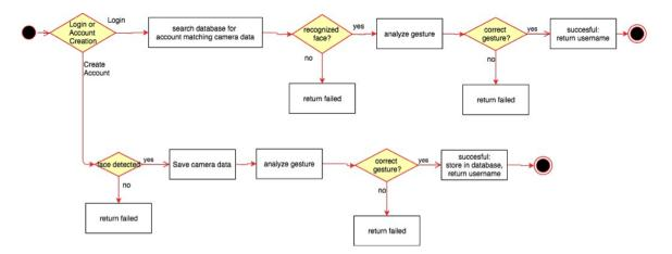
Figure 4.3: High level view of API operations
