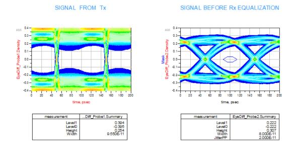
Figure 19: Layout Eye diagram
