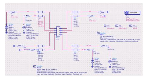
Figure 12: TDR testbench schematic [17]
