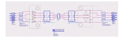
Figure 10: S-Parameter Testbench Schematic [17]
