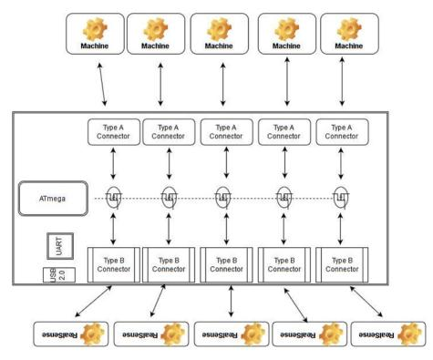
Figure 1: Interface Board Block Diagram.
