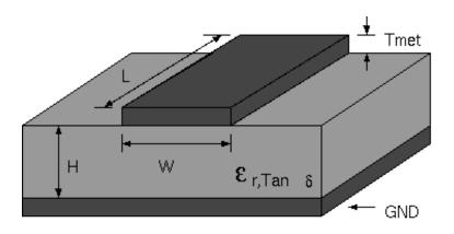
Figure 5: Cross section of a microstrip trace [10]
