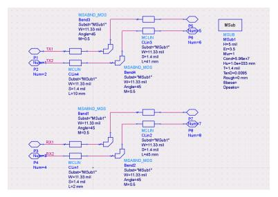
Figure 7: Modeling Microstrip Traces on PCB
