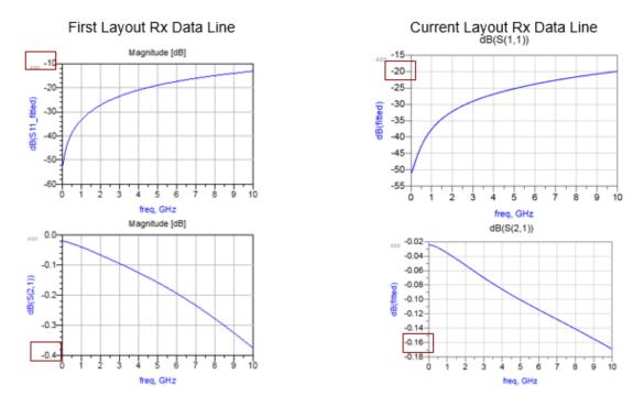
Figure 18: S Parameter Simulations
