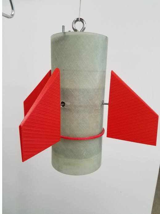
Figure 29: Payload enclosed with fiberglass coupler
