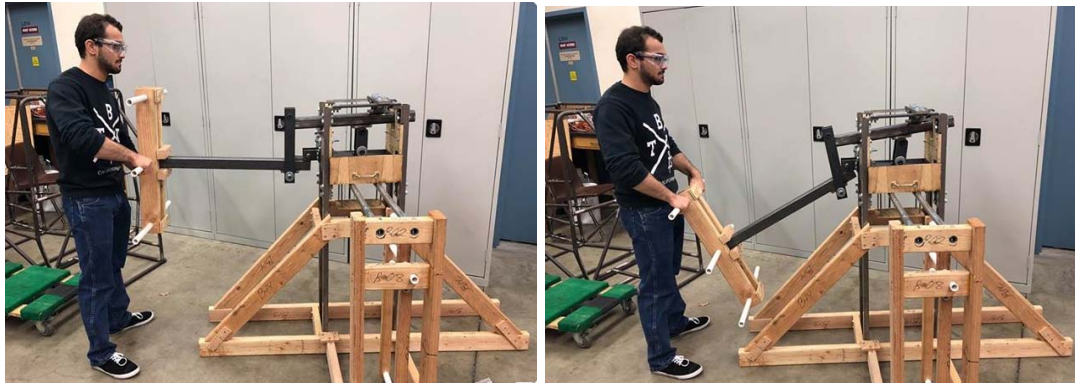
Figure 8: Step 4 of user scenario. Note that the user “climbs the ladder” when applying force on the input lever to consistently achieve maximum mechanical advantage throughout the stroke.
