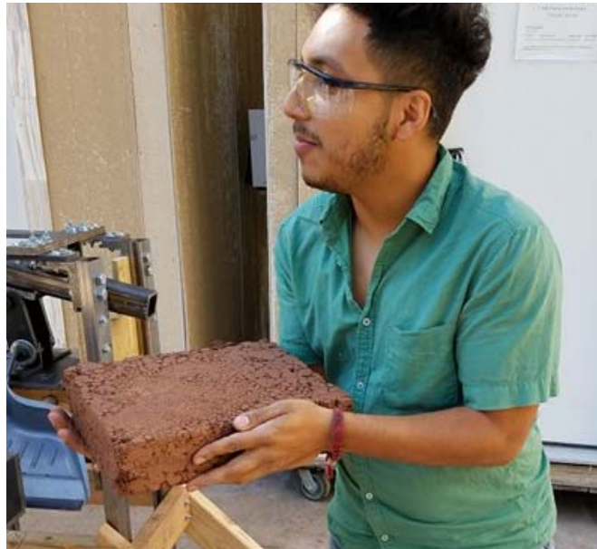
Figure 48: Compressed brick after removal from the Compression Chamber.
