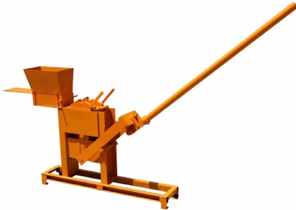
Figure 54: YLF1-40: One industry competitor for manual clay brick compression (Appendix A).
