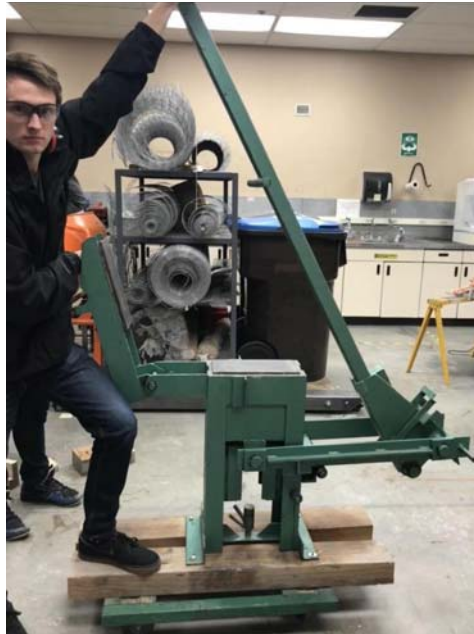
Figure 41: Picture of the makiga stabilized soil block press. The base of the chamber is completely elevated
