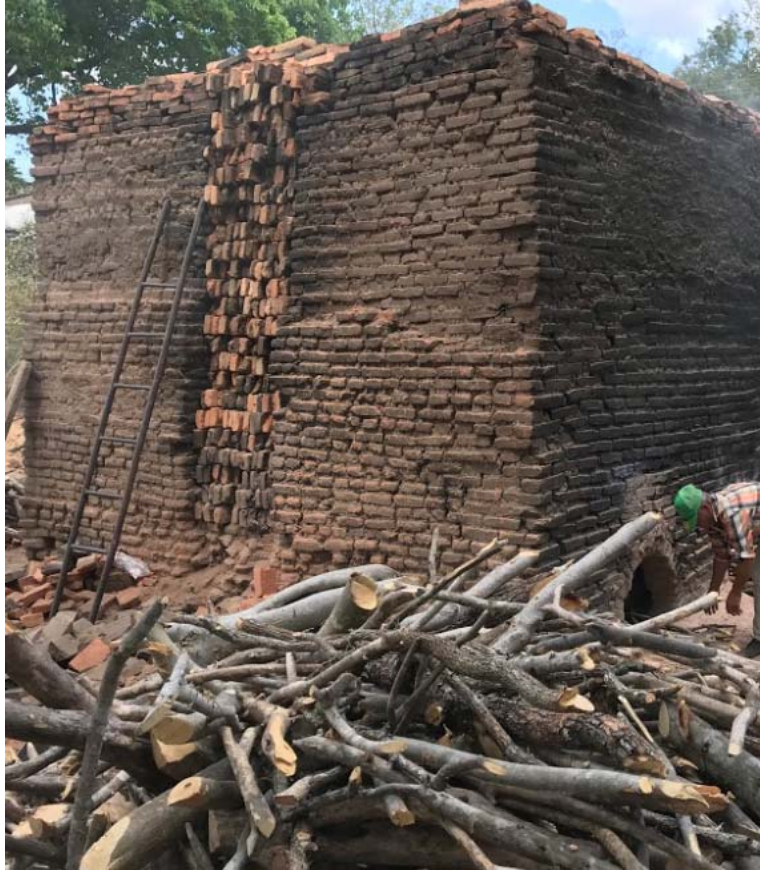
Figure 60: Clay brick oven and firewood used for baking dried bricks.
