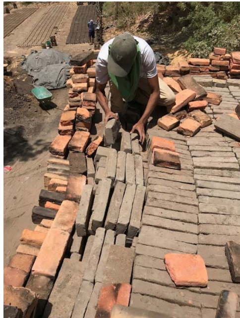
Figure 1: Clay worker in Ciudad Darío retrieving bricks from clay oven.
