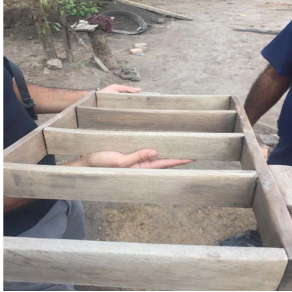
Figure 53: Wooden mold currently used to form bricks without compression in Ciudad Darío, Nicaragua.
