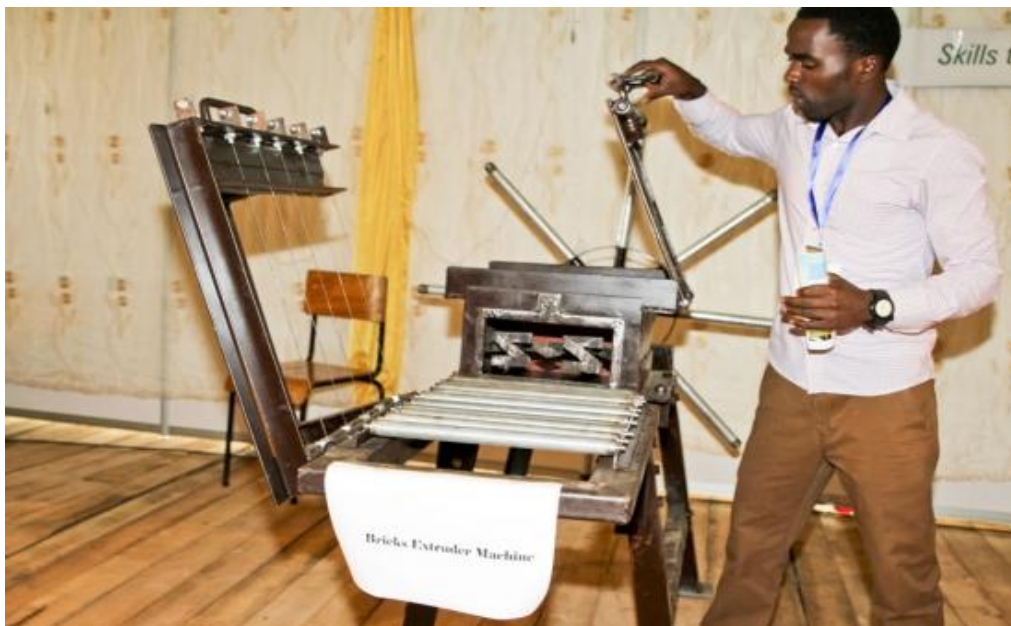
Figure 4: Brick extruder machine fabricated by IPRC -Kigali.
