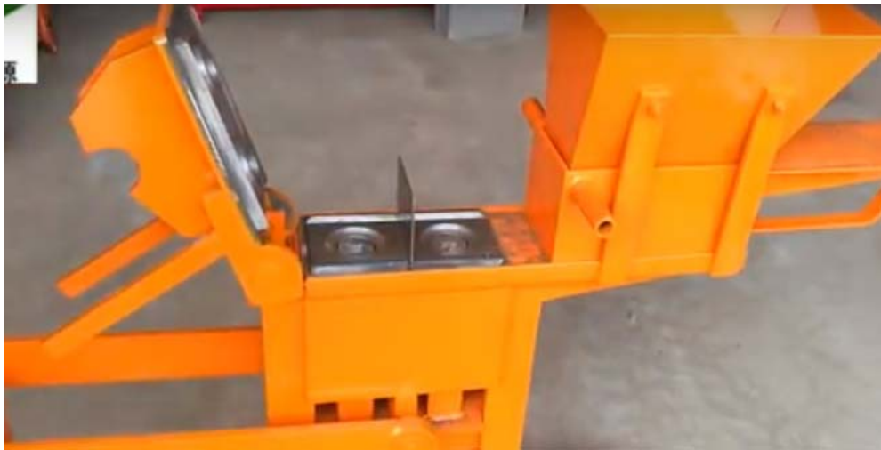
Figure 52: Removable thin metal piece of the YLF1-40 machine that allows two individual bricks to be made instead of one larger brick by allowing the brick to be cut and separated as it is being compressed. [13]
