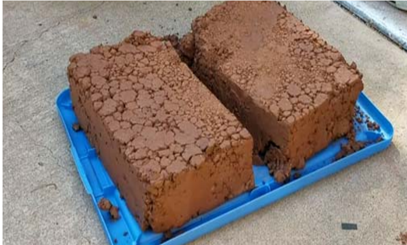
Figure 49: Double-sized brick halves after removal from Compression Chamber and being cut with sheet metal.
