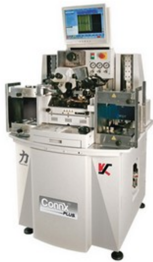
Figure 14 Kulicke & Soffa (K&S) iConn ball bonder [27].
