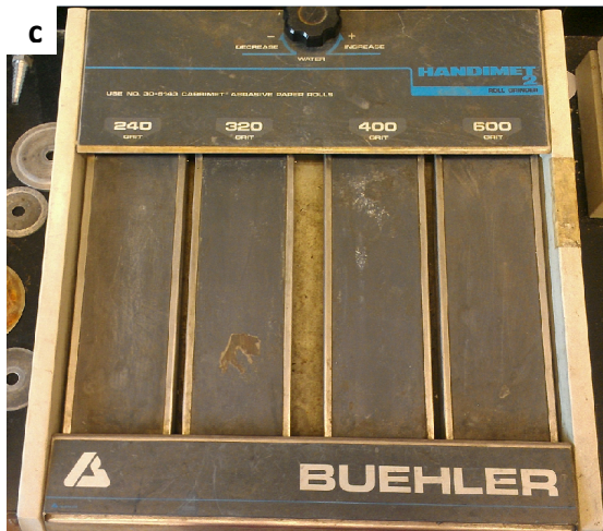
Figure 16 (a) Buehler MetaServ grinder/polisher (b) Buehler Isomet 1000 Precision cutter (c) Buehler Handimet 2 Roll Grinder [28].
