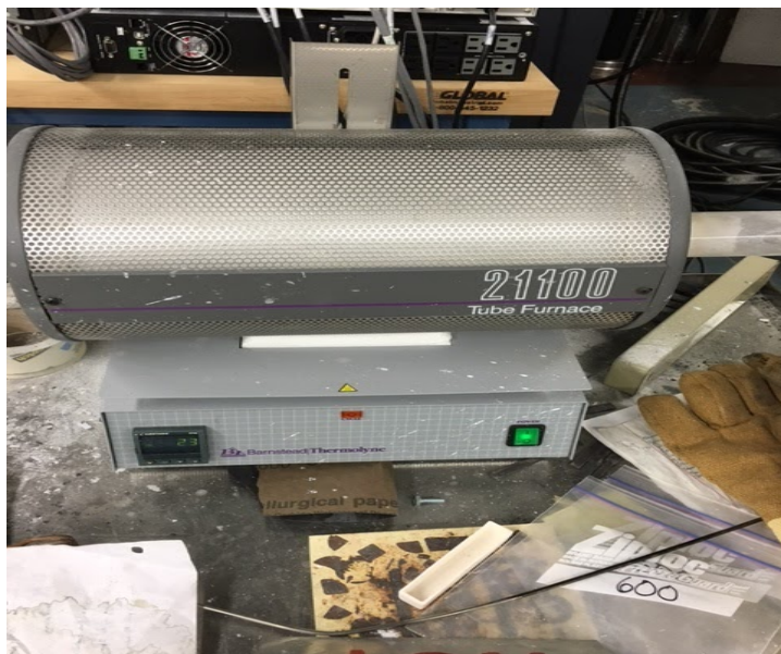
Figure 17 Heating Tube Furnaces.
