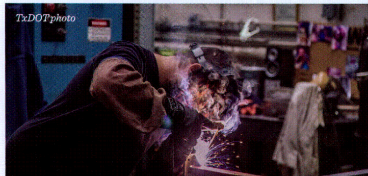
Daniel Wilson, metal fabrication specialist, finishes up the welding and fabrication of an arrow board mount for a new large herbicide truck build.
