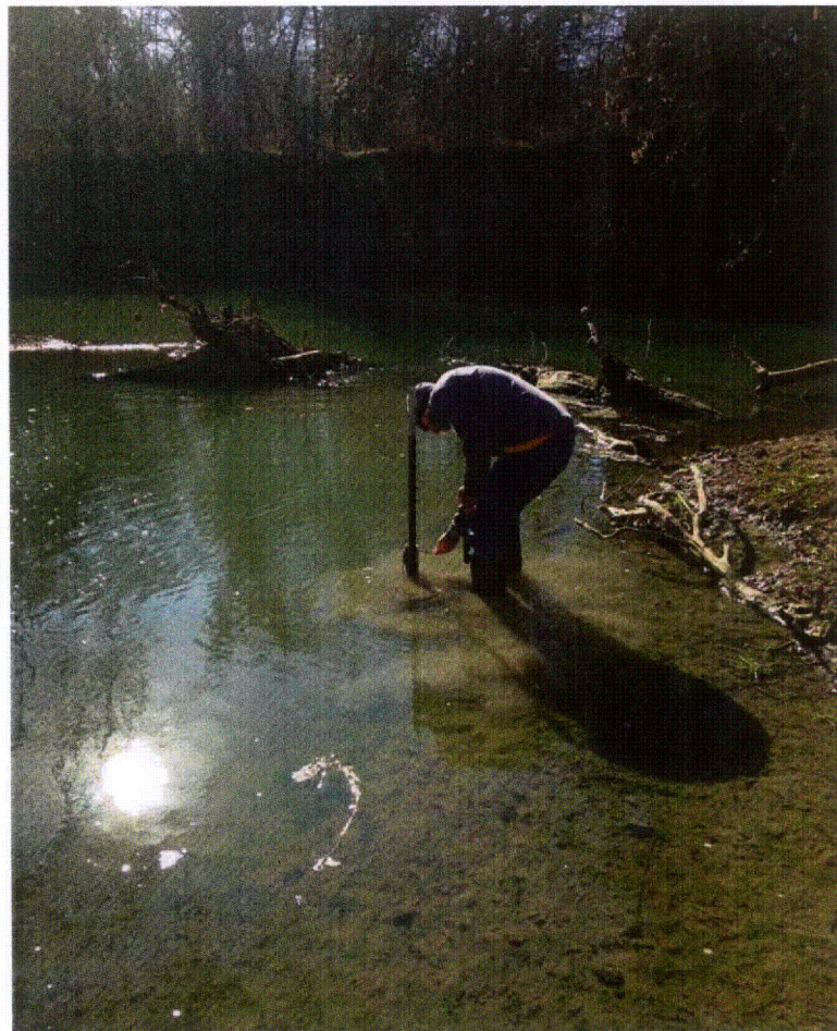
Figure 10. Crew member installs a stream level logger.
