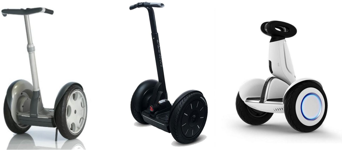
Figure 3. Evolution of Segway Devices over Time: 1st Generation, 3rd Generation, Smaller Variant
