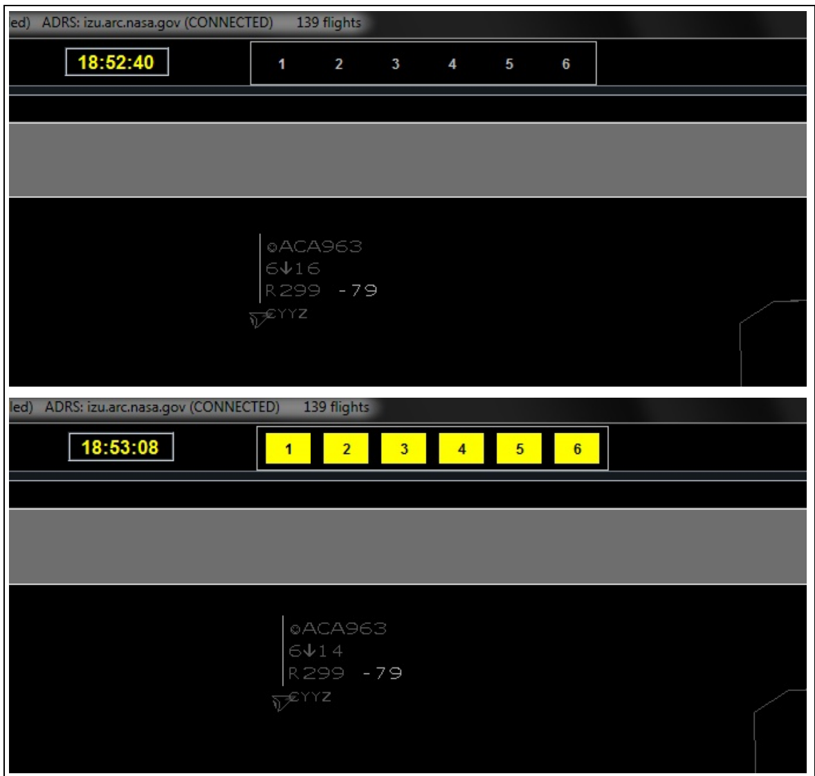
Figure 5. Example of the Air Traffic Workload Input Technique (ATWIT) implemented in MACS.
