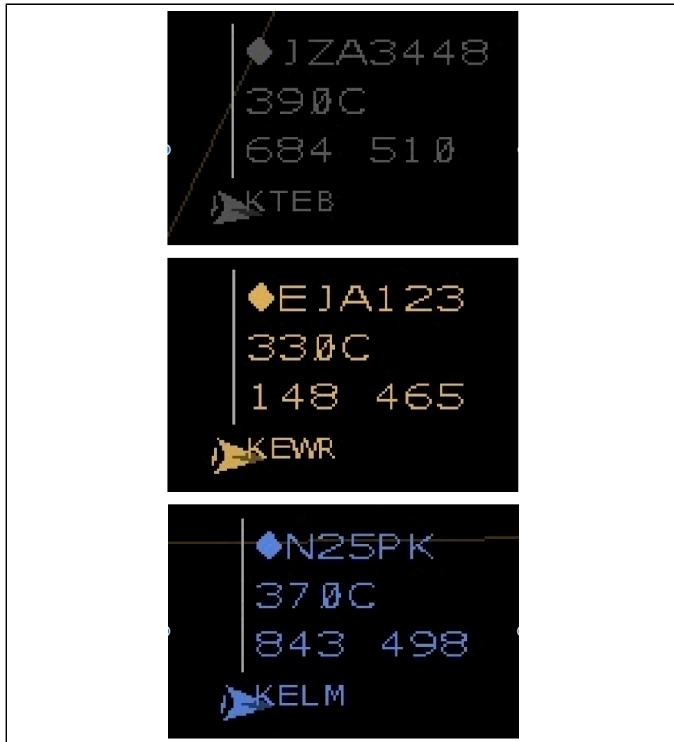
Figure 4. Example of aircraft color changes according to command used. From top to bottom: Top – Nominal aircraft color. Middle – MM command used. Bottom – AA command used.
