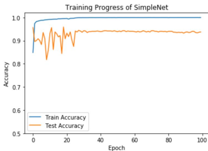
Figure 13 Training Progress of SimpleNet with Augmentation: After augmenting the dataset, there was a substantial improvement in the SimpleNet model. Even early on, the test dataset accuracy bounces from 80% to around 95%. Although it was initially unstable, the model stabilized right around epoch 30.
