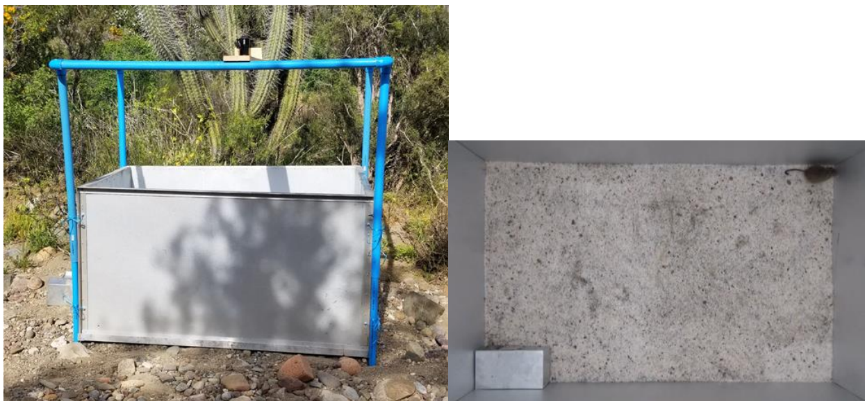
Figure 2.3 Left: open field box in situ with tetrapod (in blue) to hold video camera in place. Right: still image from video of behavioral trial. The box in the lower left corner of the OFB served as a hide for subjects, to which they acclimated for 3 minutes and, once opened, could return to for shelter
