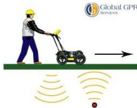
Figure 1 A graphic illustrating the basic principle of GPR
