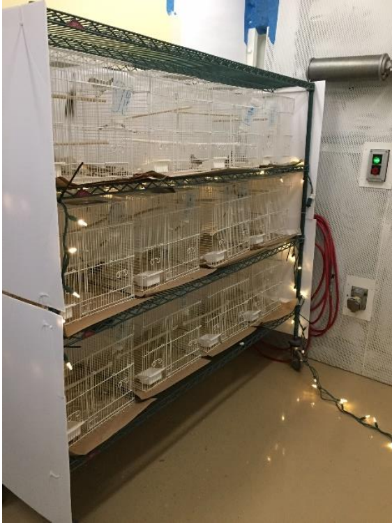
Figure 2.1 Cages set up in the plenum of the hypobaric climatic wind tunnel. Lights were added to provide additional lighting to bottom cages. Each cage on the rack housed an individual bird during the experimental manipulations, and identical cages and racks housed individual birds in their home rooms.
