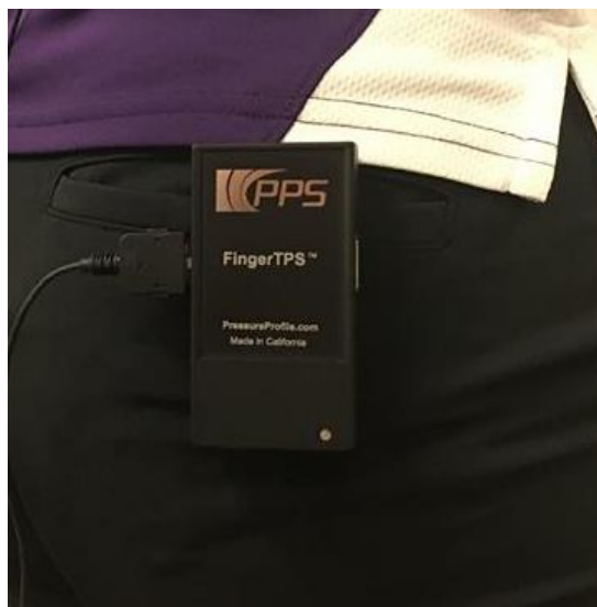
Figure 24: The rechargeable electronic interface module (D710 interface) attaches to a belt or the waistline of the participant's pants and is responsible for transmitting the data collected by the finger sensors to the computer through Bluetooth.
