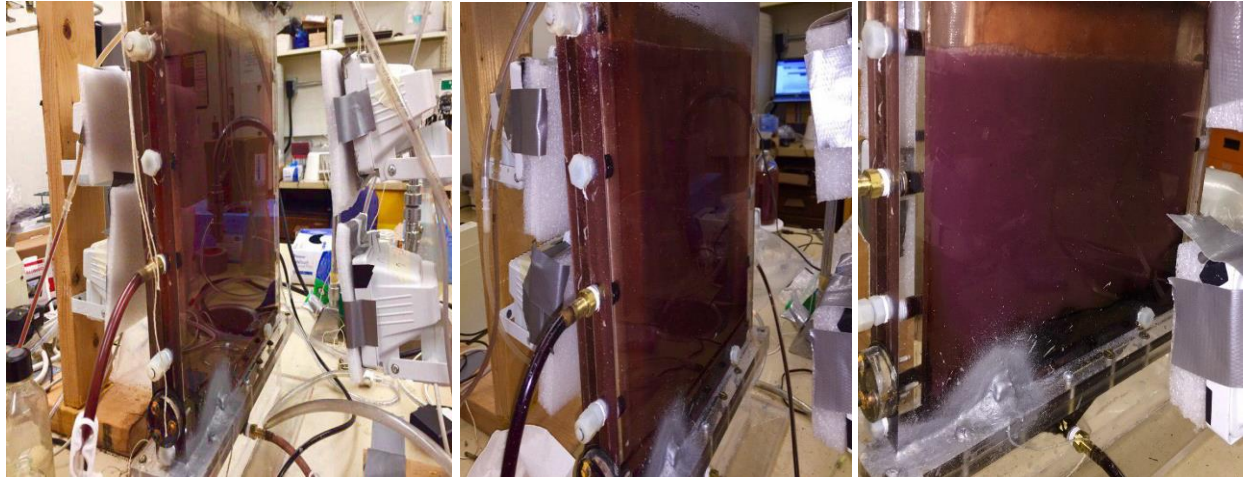
Figure 4.1. Continuous membrane photobioreactor configuration at 3 Wm -2 (left), 1.4 Wm -2 (center) and light-dark cycles of 2 h-2 h at light intensity of 1.4 Wm -2 (right)
