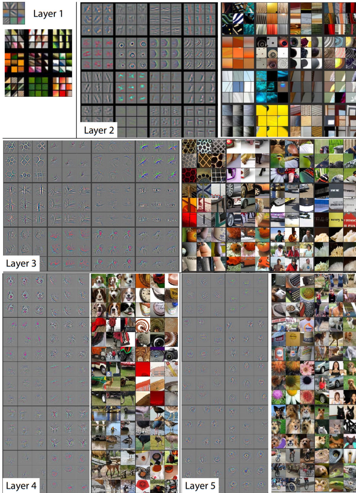
Figure 2.12: Visualization of each layers from 1 to 5 of a modified AlexNet [26]. The original images are to the right of the kernel blocks.
