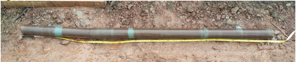
Figure 35. Run 10 from elevation 95.2 to 93.7m.
