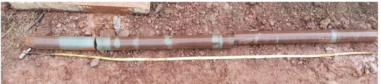
Figure 32. Run 7 from elevation 99.9 to 98.4m.
