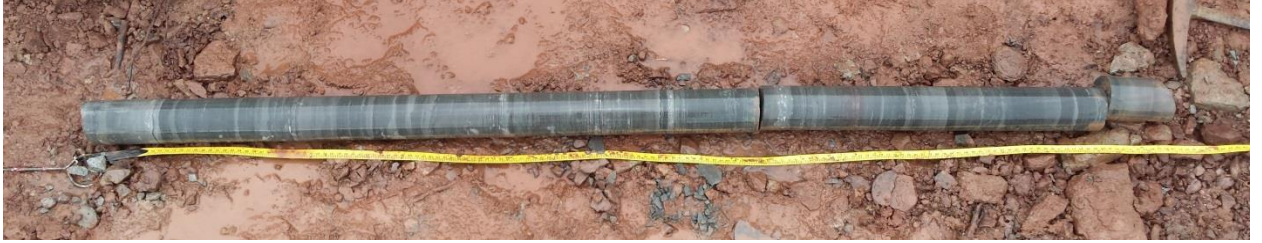
Figure 25. Run 24 from approximate elevation 63.0 to 61.5m.
