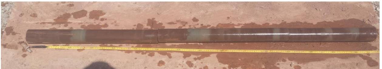
Figure 59. Run 13 from approximate elevation 83.0 to 81.5m.
