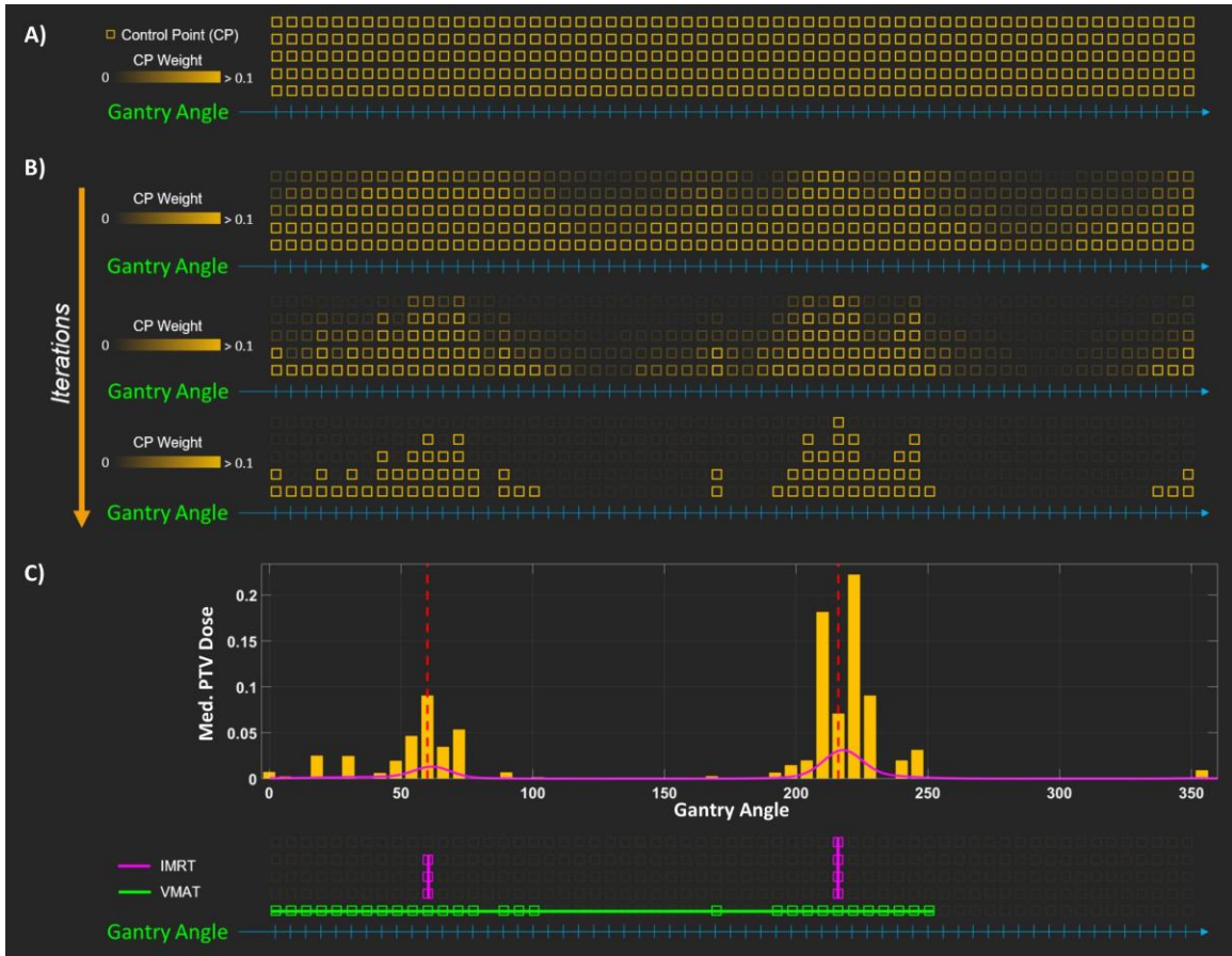
Figure 6.2: Illustration of the new UIMAT algorithm. A) FMO and aperture sequencing (each CP illustrated as a square) is performed at 4^\circ increments. B) DAO with a CP weight regularizer is performed. As this DAO progresses, the regularizer eliminates CPs from the treatment plan. C) The results of this DAO are parsed and VMAT (green) or IMRT (purple) beams are sequenced using the CPs from B). A final DAO is then performed.
