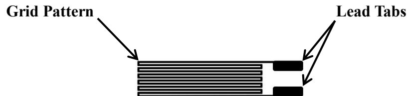
Figure 1.12: Strain Gauge Schematic
