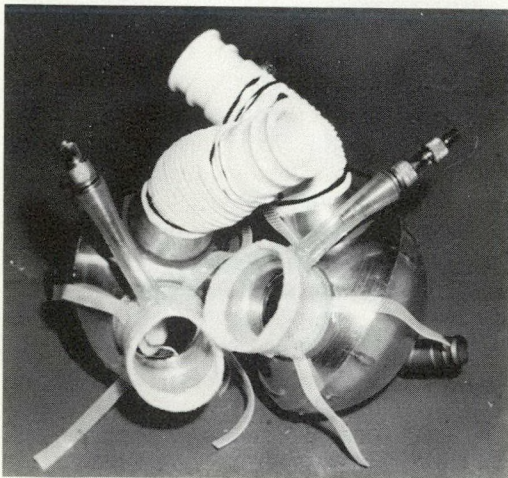
Fig. 2.—Each side of the artificial heart is separate and weighs 135 g. Dacron graft arteries and atria simplify anastomosis to the natural vessels.
