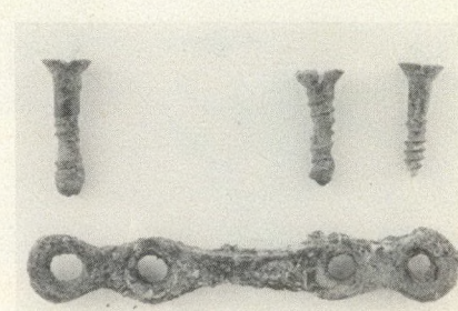
FIG. 2—Lane plate and screws after removal from bone (original magnification \times 2.5 ).
