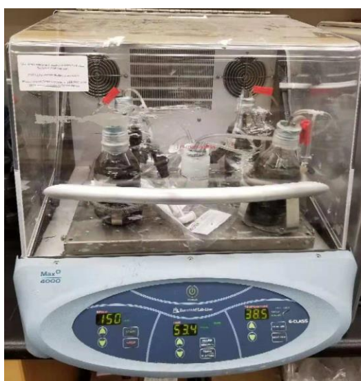
Figure 4-1: The set-up of anaerobic digestion batch test.
