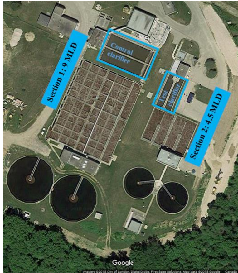
Figure 3-1: Lay out of Vauxhall WWTP.
