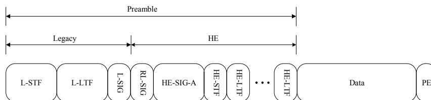
Figure 2.5: Format of HE TB PPDU
