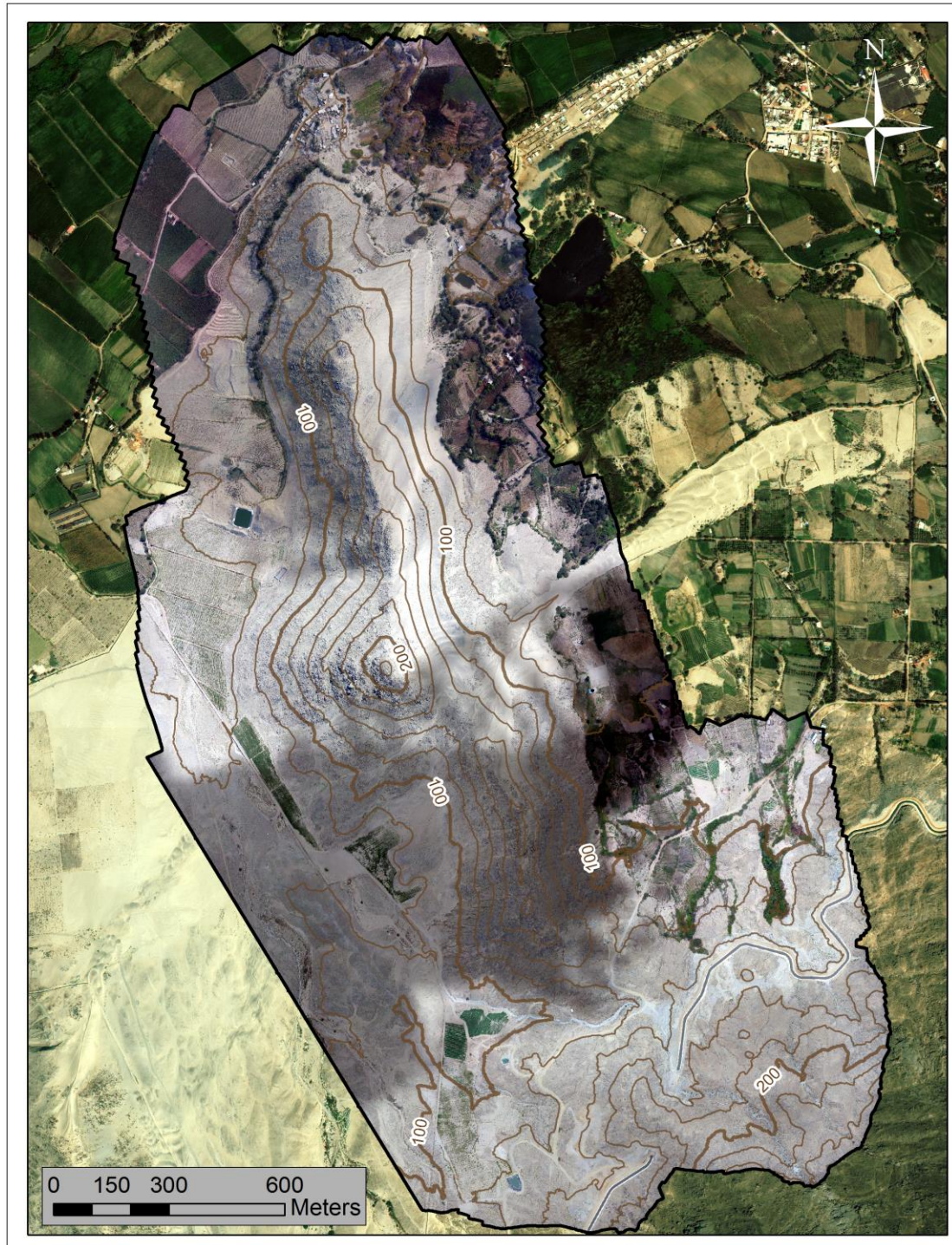
Figure 3.4: Final post-processed orthophotograph covering 3.81 km 2 of Cerro Arena and its environs (georeferenced image included as supplementary information). Contours extracted from DEM and set at 20 meter intervals.
