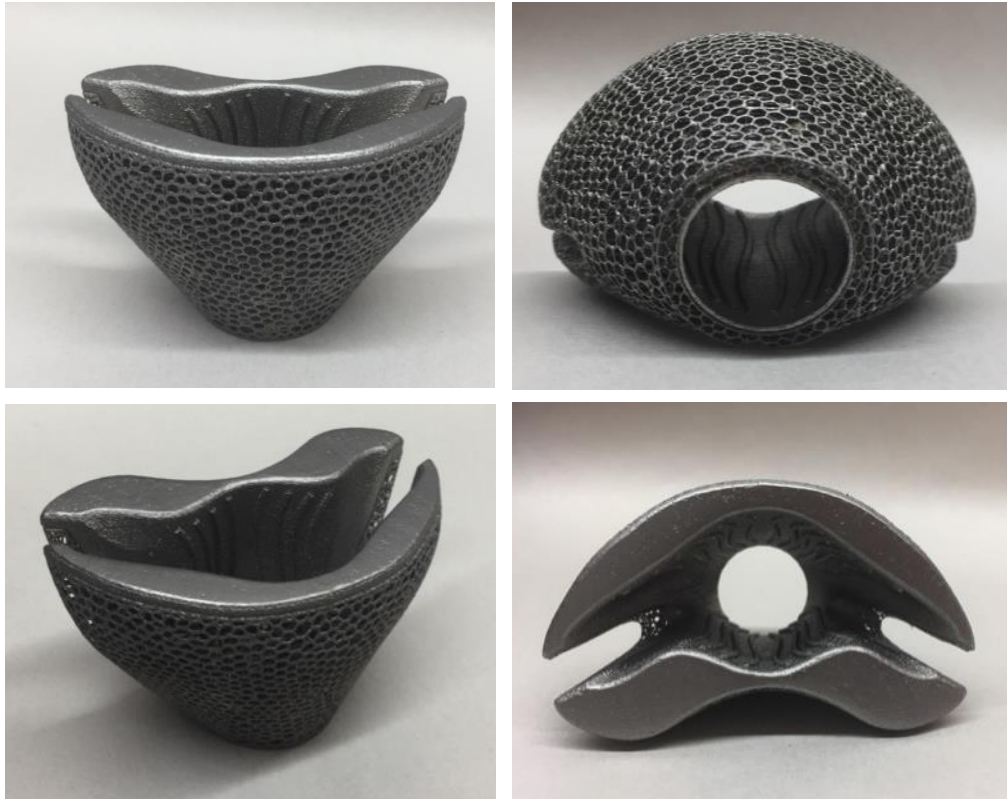
Figure 5.4. Novel 3D printed titanium revision TKA augment for the proximal tibia.
