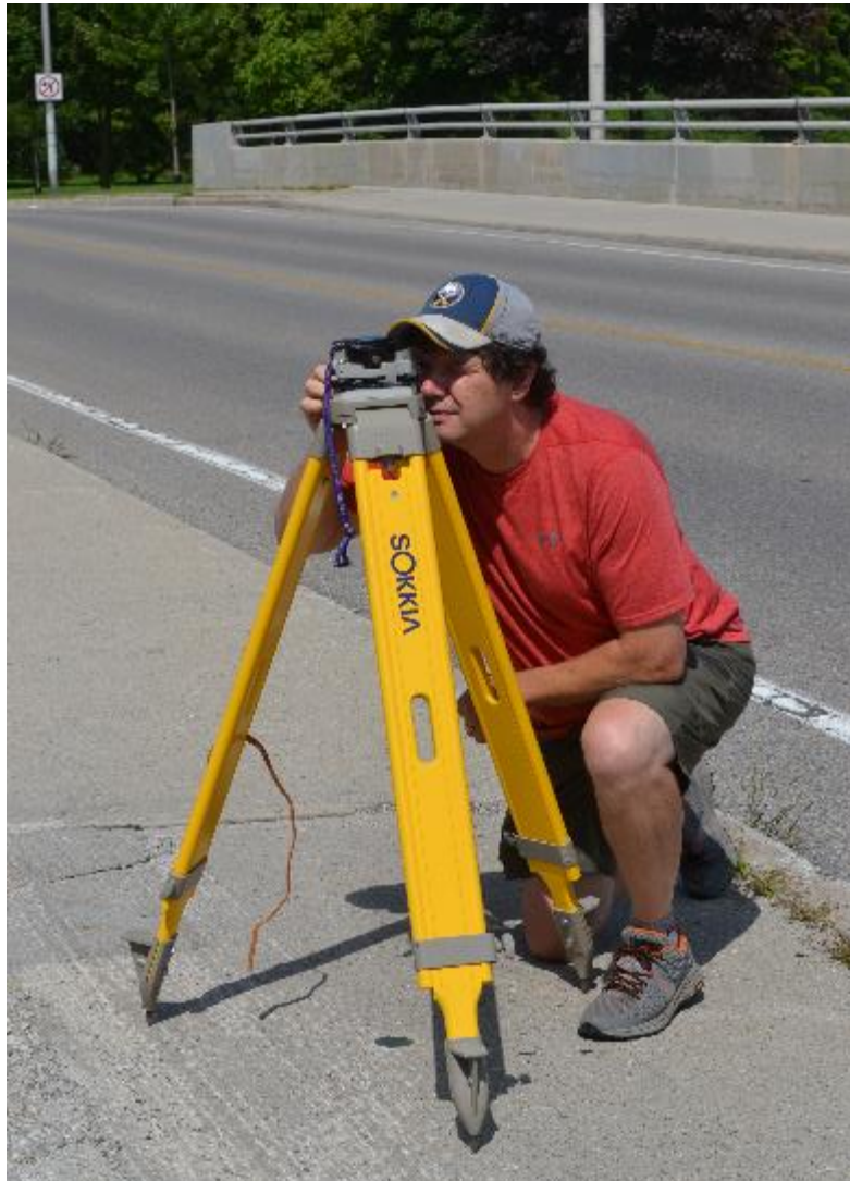
Figure 4.5: Author aligning surveyor tripod over horizontal survey monument
