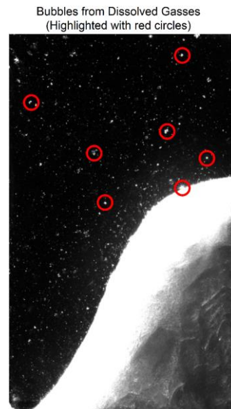
Figure 8: Highlighted bubbles from dissolved gasses during lauric acid melting
