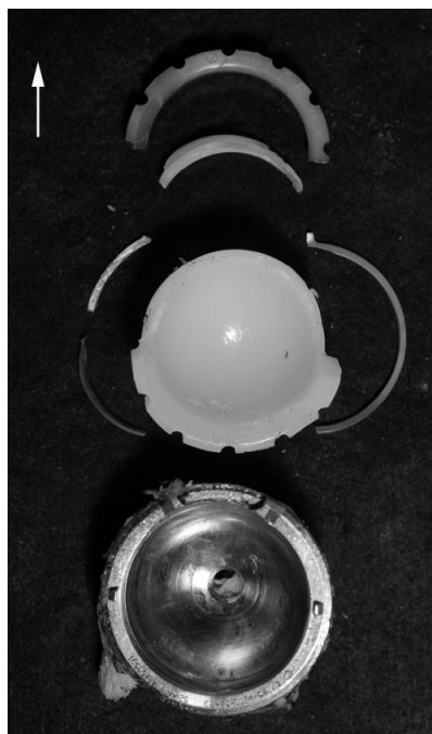
Figure 2-4 - Example of a retrieved fractured remelted HXLPE liner at the implant rim. (Permissions from Moore KD, Beck PR, Petersen DW, Cuckler JM, Lemons JE, Eberhardt AW. Early Failure of a Cross-Linked Polyethylene Acetabular Liner: A Case Report. J Bone Joint Surg Am. 2008;90(11):2499-2504. doi:10.2106/JBJS.G.01304)
