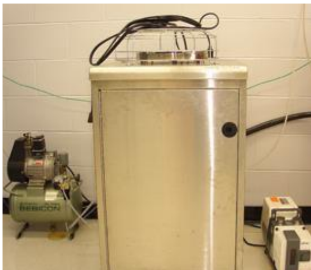
Figure 3.1. Savannah 100 ALD system (Cambridge Nanotech, USA)
