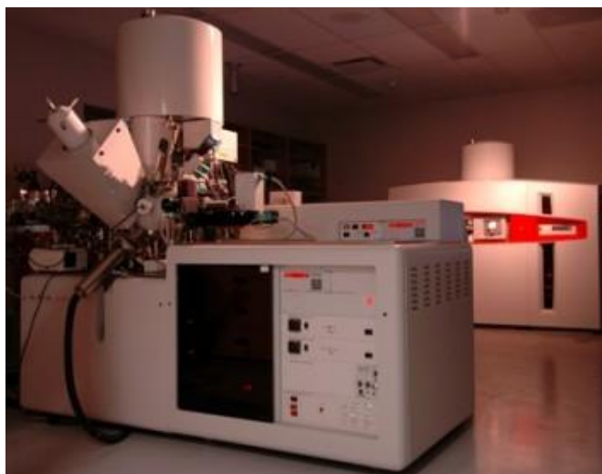
Figure 3.6. A Krato AXIS Ultra Spectrometer XPS.
