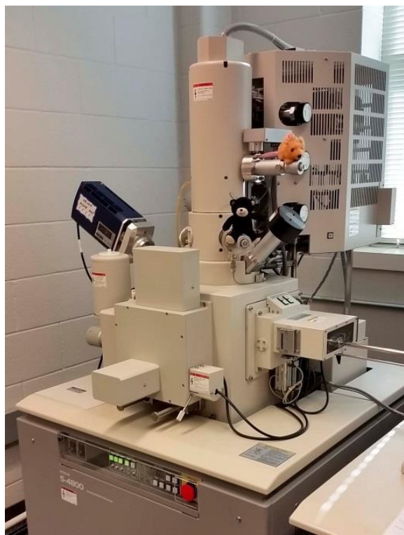
Figure 3.4. Field emission scanning electron microscope (Hitachi S-4800).
