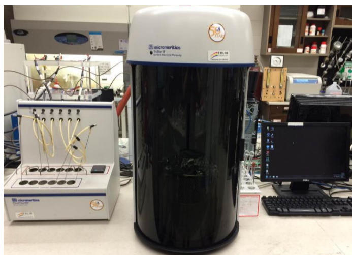
Figure 3.8. Micromeritics TriStar II 3020 Surface Area and Pore Size Analyzer
