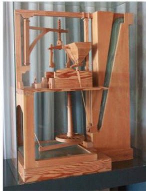
Figure 5.5: Scale model of a water-powered flourmill in the “Water Systems” room. With it, an explanation of Al-Jazari’s 33 contributions to the mechanics of hydraulic mills (6 July, 2010; photo by author)
