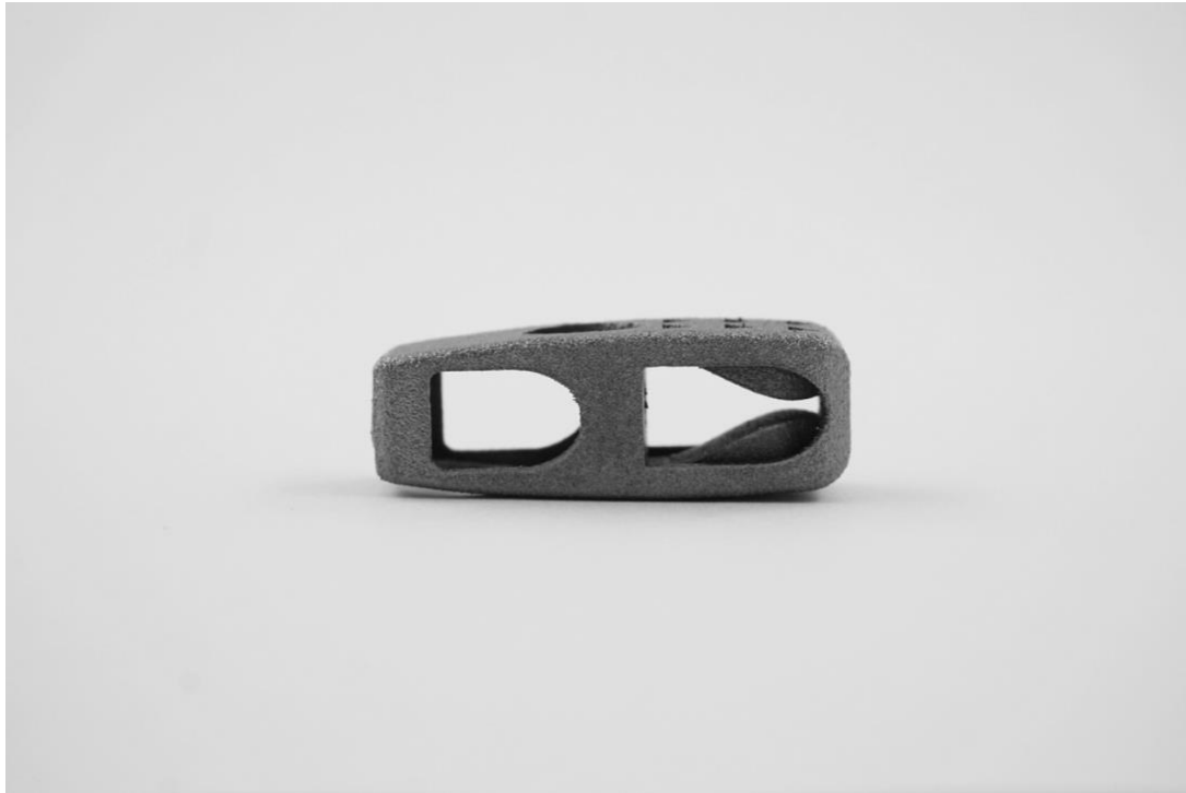
Figure 3-6: Lateral view (photograph of actual cage) of stand-alone cage for posterior interbody lumbar fusion.
