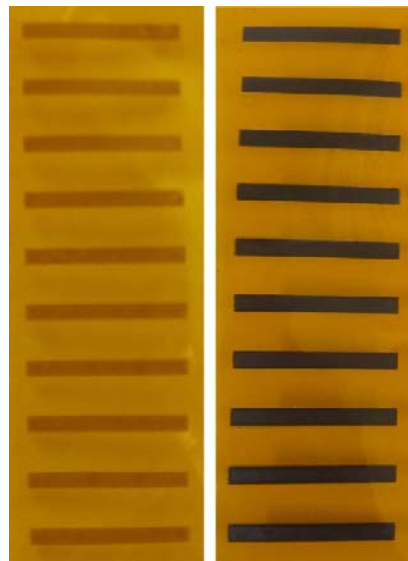
Figure 5.2 Ribbon GO electrodes before (left) and after (right) annealing. Electrodes lose their transparency due to removal of oxygen containing groups during thermal reduction process (Sinar, Knopf, & Nikumb, 2014).
