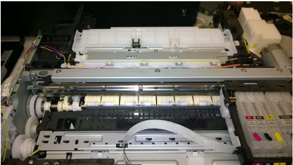
Figure 4.1 Paper feed mechanism of a Canon IP7220 inkjet printer. Office inkjet printers feature rollers to feed paper through and keep it in place during printing process. Regardless of feeding route, paper goes through rollers after inkjet printing.
