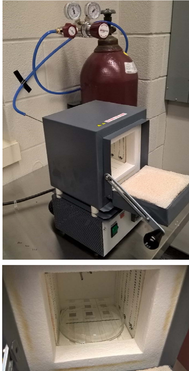
Figure 5.1 Muffle furnace setup used for this research. Argon gas was supplied during treatment to remove oxygen from the furnace chamber.
