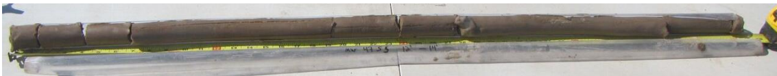
Figure A.12 EK-Bio MW1 location core from 3.66 m to 4.27 m showing homogenous low plasticity brown clay. MW1B screened interval is 3.66 m to 4.27 m bgs
