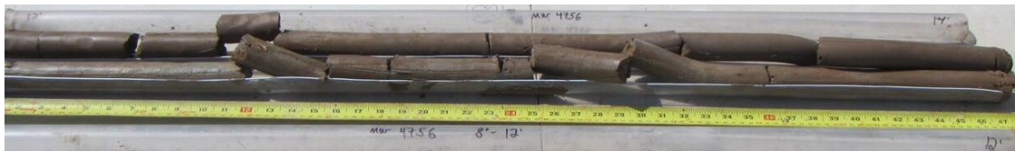
Figure A.13 EK-Bio MW2 location cores showing homogenous low plasticity brown clay in 2.44 m to 3.66 m interval (bottom) and 3.66 m to 4.27 m interval (top). MW2A screened interval is 3.05 m to 3.66 m bgs and MW2B screened interval is 3.66 m to 4.27 m bgs.
