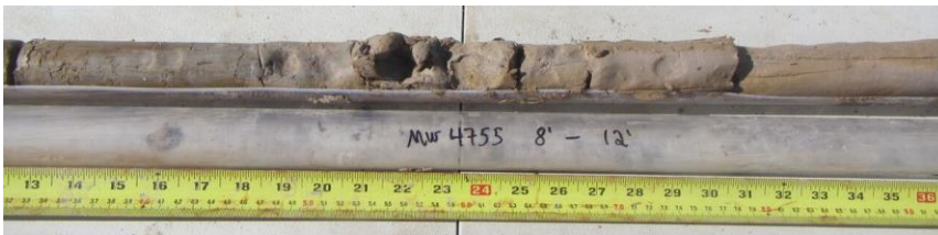
Figure A.11 EK-Bio MW1 location core from 2.44 m to 3.66 m showing distinct visual differences from the low plasticity brown clay seen at other EK-Bio monitoring locations. This is evidence for a potentially higher permeability layer due to some silt and sand within a higher plasticity clay. MW1A screened interval is 3.05 m to 3.66 m bgs.
