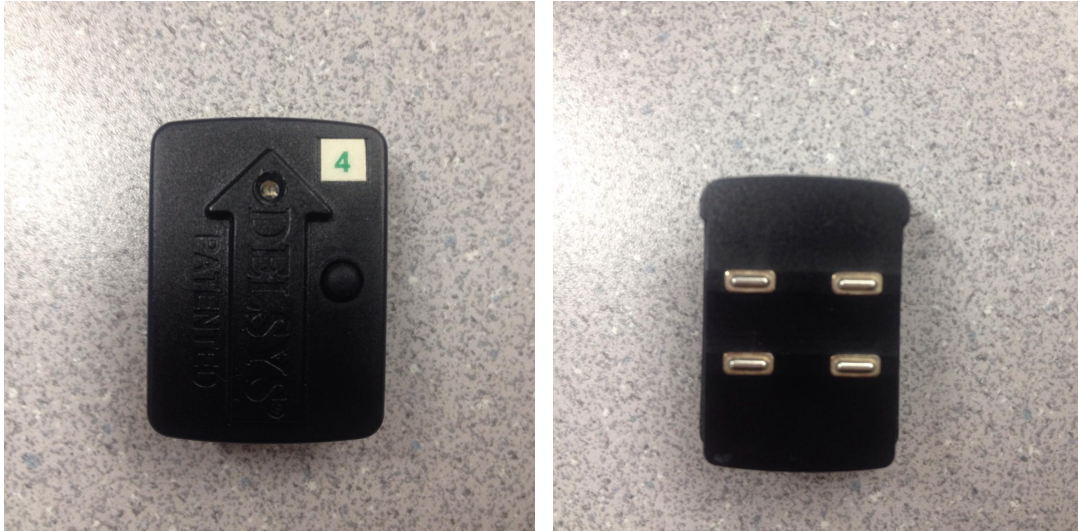
Figure 3.2: Trigno sensor. The front of the sensor (left) includes an arrow to assist with the direction of sensor placement. The arrow should be aligned in the direction of the muscle fibres. The x axis of the accelerometer is parallel to the sensor arrow, and y axis is perpendicular and coplanar to the sensor arrow. The back (right) of the electrode contains 4 bar electrodes.
