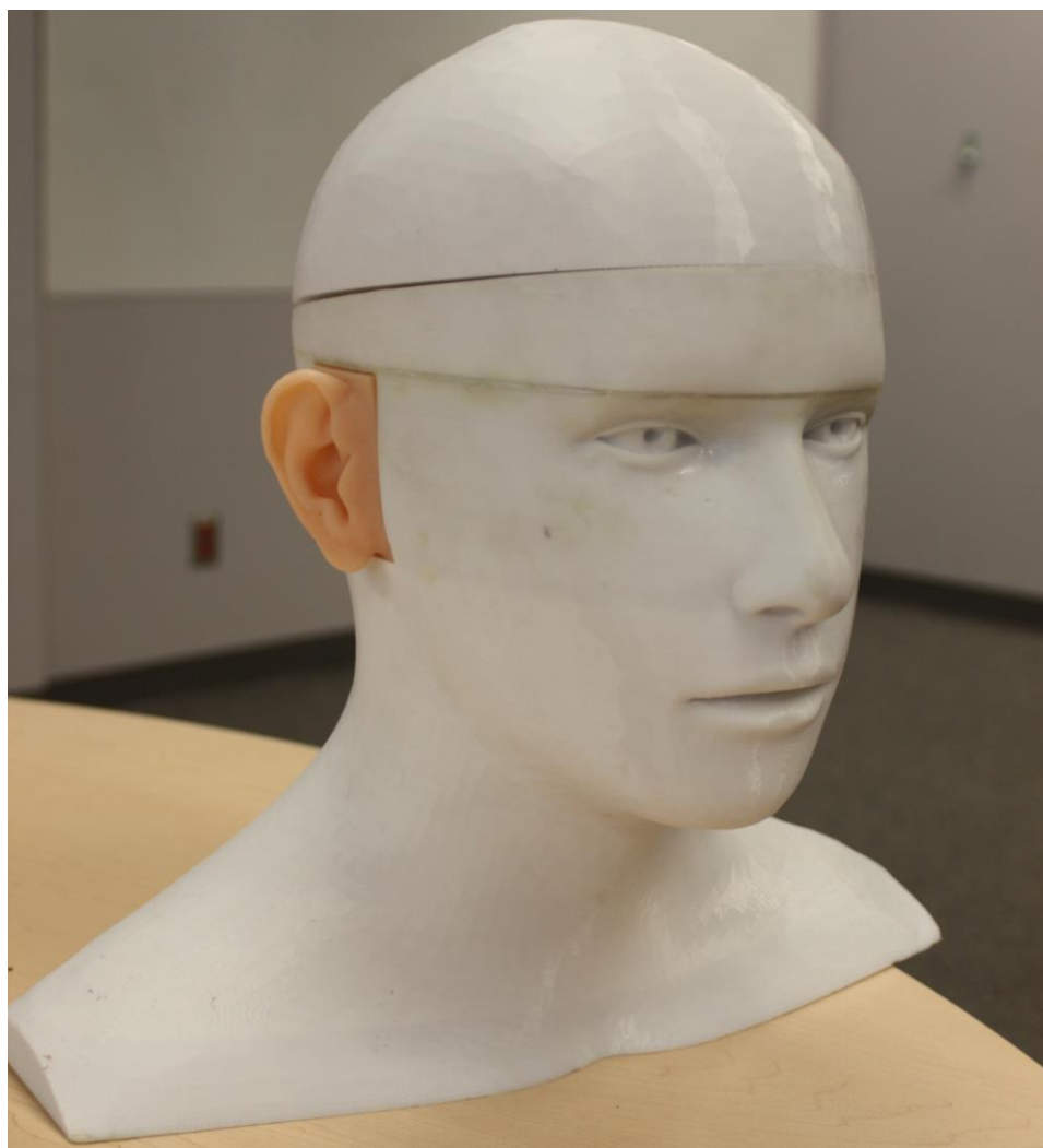
Figure 4.1: The updated simulator showcasing the new flexible silicone ear and the fully 3D printed head model.
