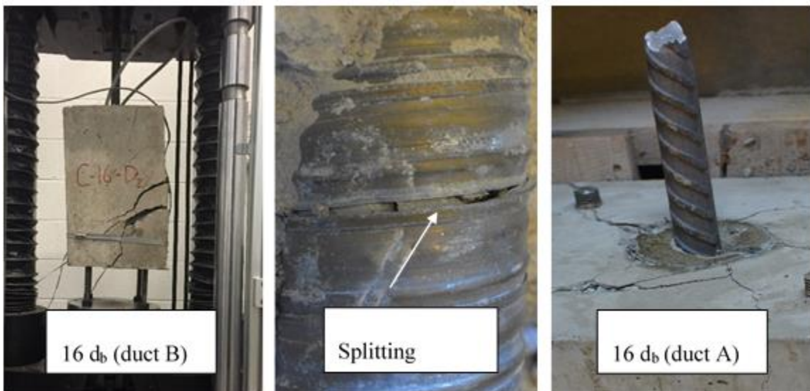
Figure 5.9: [Left] Duct rupture (C-16-D2); [Center] Expanded grout as confinement is lost (C-16-D2); [Right] Additional confinement causing bar fracture (C-16-D4).
