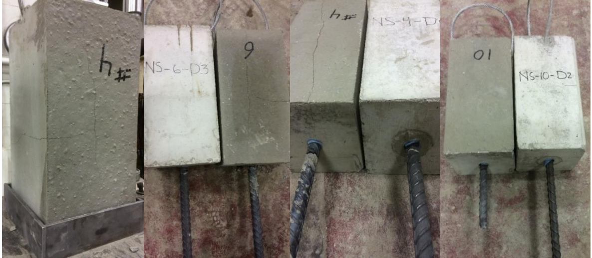
Figure 4.6: (left to right) Split tensile cracking (C-4-D1); Pull-out failures vs splitting failures of comparable specimens at 6 and 4 db (NS-6-D1/ C-6-D1 and C-4-D2/ NS-4-D1, respectively); and Slippage of bars vs bar fracture at 10 db embedment (C-10-D2 and NS-10-D2).
