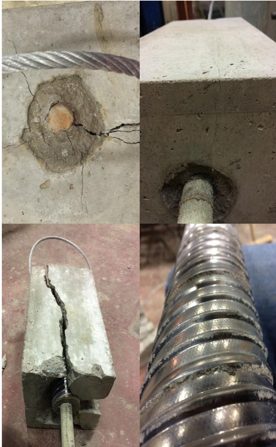
Figure 3.5: [Top Left] Splitting failures in ductless Grade 60 at 12 d_b (NS-12-D1-ND); [Top Right] Splitting cracks between duct and concrete block (NS-12-G1); [Bottom Left] Duct pull-out (NS-12-G2); [Bottom Right] Failed cones between duct ribs (NS-12-G2).
