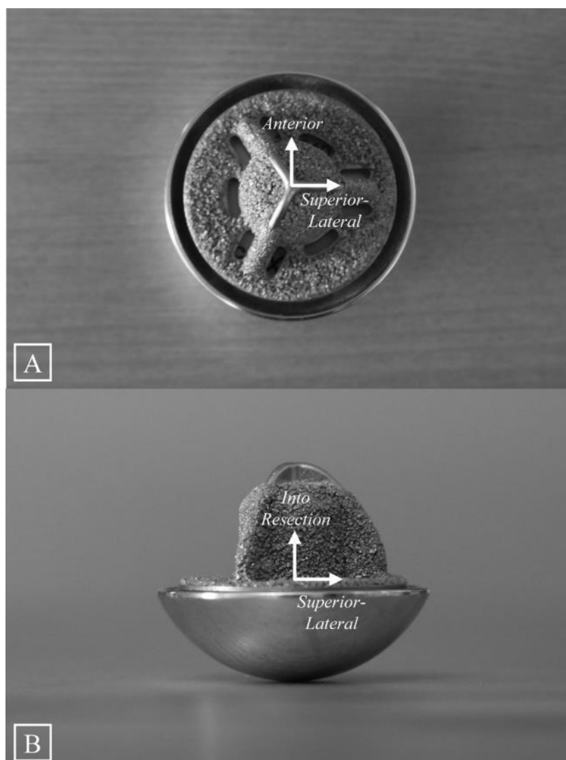
Figure 2.2: Stemless Relevant Cartesian Coordinate System As an example, the Tornier Simpliciti implant is presented to demonstrate that a stemless implant-relevant Cartesian coordinate system should be constructed with axes directed (A) superior-laterally, anteriorly and (B) perpendicular to the underside of the implant.
