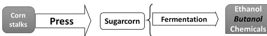
Figure 6.1. Flow diagram of sugar extraction from corn stalks juice for biobutanol production
