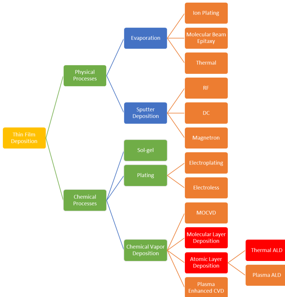
Figure 1.1. Family tree diagram of common thin film deposition techniques [4]. Processes central to this thesis are highlighted in red.
