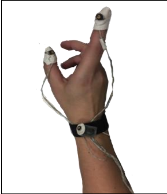
Figure 4. Participant's hands with IRED sensors attached to the thumb, index finger and wrist.
