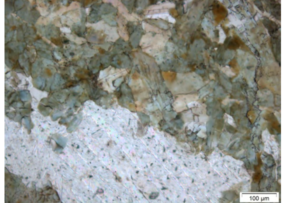
Pyrite rich vein margin with tourmaline, sericite with rutile inclusions and interstitial gold (5X RFL)
