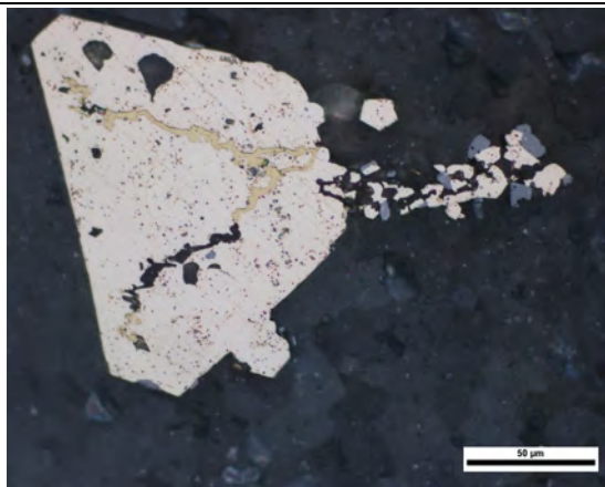
Subhedral, inclusion rich pyrite grain with chalcopyrite and rutile (50X RFL)
