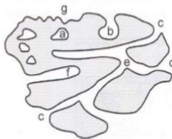
Figure 2.15 Schematic Representation of a Porous Solid, Showing the Most Common Types of Pores: a: closed pores, b,c,d,e,f : open pores, b,f: blind pores, e: through pores
