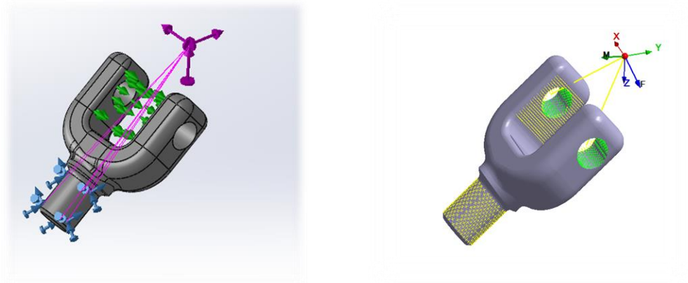
Figure 3.4: Boundary conditions of humeral yoke
