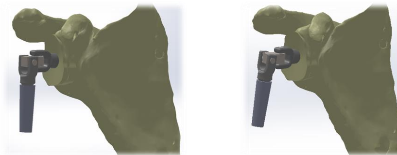
Figure 2.7: Offset distance of hinge joints in center trunnion variation
