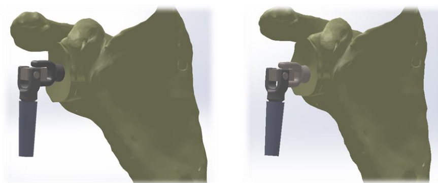
Figure 2.5: Glenoid yoke position variation
