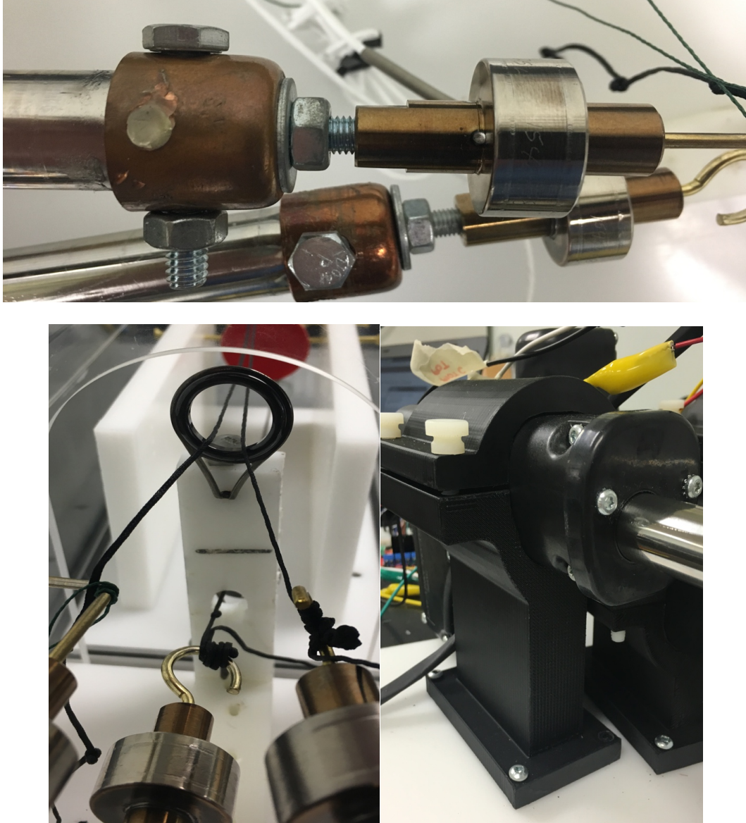
Figure B.3: Cap, Rod Guide, and Motor Mount
