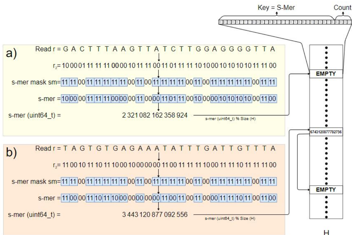
Figure 3.4: Data Structure 1: S-Mer Insertion. An overview of how s-mers are inserted. a) A s-mer is inserted with a key 2 321 082 162 356 924 finding an empty spot in H . It is inserted, where the first 28 bits contain its s-mer, and the last 8 bits contain its count. b) A s-mer is inserted with a key 3 443 120 877 092 556 and encounters a collision. It will then use double hashing to find another empty spot in H .
