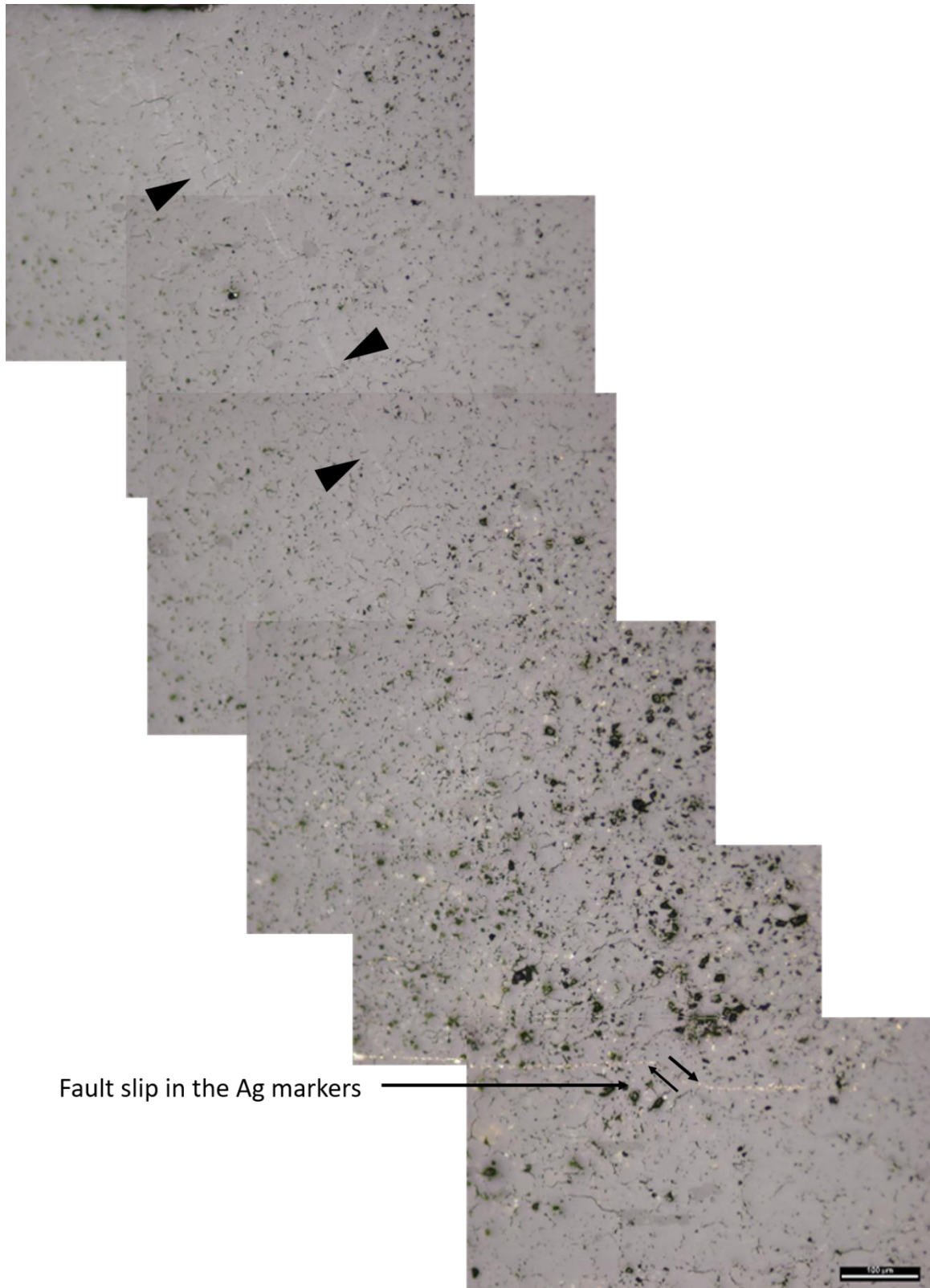
Figure 7.33: Composite micrograph in reflected light of \sim 1/3 of the length of a fault that traverses the entire length of HPF_AE_15. In the N-W region of the image ahrensite can be seen as thin bright line contained within the fault zone (black arrowheads), but eventually disappears about 1/4 of the way along the rupture. Further along the fault in the bottom panel the Ag marker has been displaced as indicated by the black arrows.
