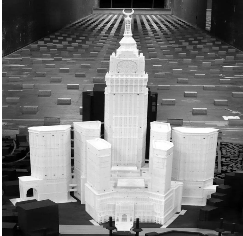
Fig. 2- 6: Pressure test model tested at the BLWT (Boundary Layer Wind Tunnel report, 2008)
