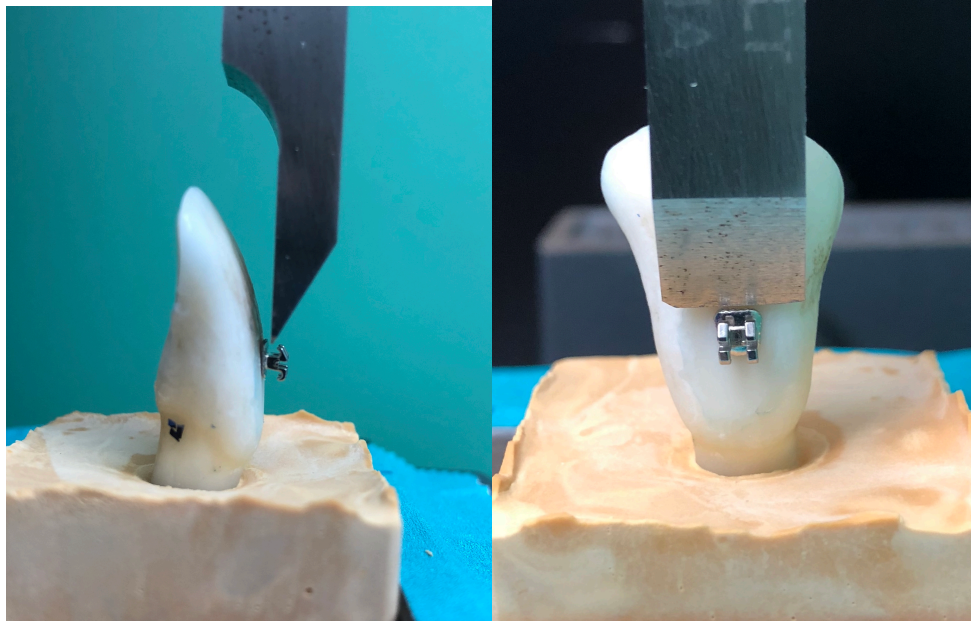
Figure 20. The instron blade is positioned above the bracket.
