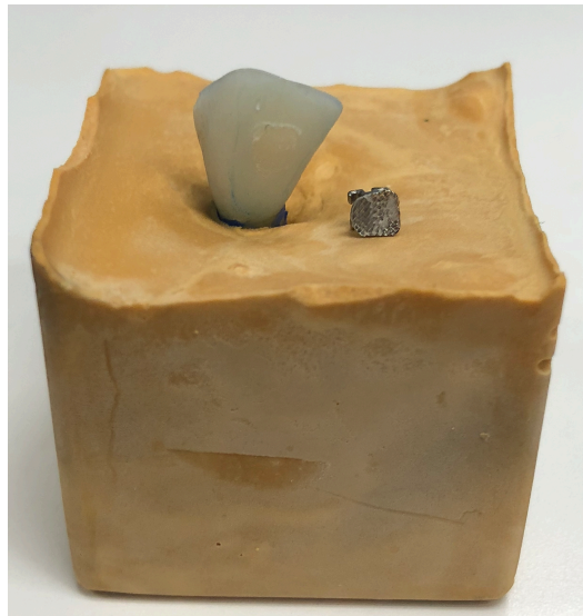
Figure 22. Mounted tooth with de-bonded bracket.
